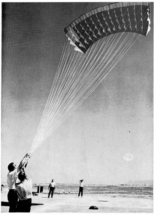
KITE-LIKE, a Para-Foil is launched by Division 9324 personnel during a test in Coyote Test Field. The system when tethered with a cable provides a stable "sky-hook" for instrumentation cables. In free flight, the Para-Foil is combined with an automatic homing system which brings rocket payloads down to a ground station transmitter.
